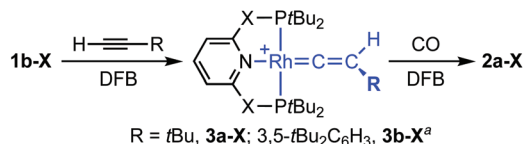
Scheme 3 Preparation of vinylidene complexes 3 ( \text{X} = \text{O}, \text{CH}_2 ). [\text{Bar}^{\text{F}}_4]^- counter anions omitted for clarity; a 3b-O formed as mixture with the corresponding \pi -complex 2e-O .
