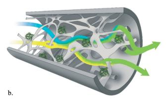
Fig. 1 Portrayal of mixing and homogenization intensity in laminar flow (a) and in (micro)structured monolithic reactor (b).
