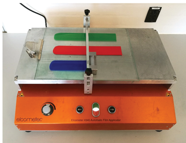
Fig. 10 Casting of thin silicone elastomer films, using a commercial film applicator and knife. The bar across the plate can be set to move at different speeds. The knife can be varied in length and gap. Some knives have built-in chambers for the liquid to be coated.
