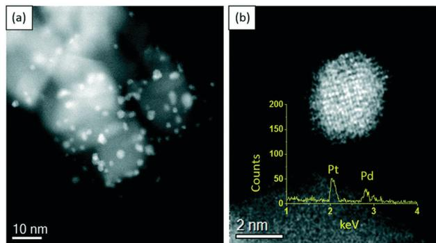
Fig. 27 Scanning transmission electron microscopic images of Pd–Pt/ $\text{TiO}_2$  catalyst at different magnifications. The formation of random Pd–Pt nanoalloys is confirmed from the Z-contrast high-angle annular dark-field imaging and the X-ray energy-dispersive spectrum (inset image, b) taken from an individual particle. Reproduced with permission from ref. 336. Copyright (2018) Royal Society of Chemistry.
