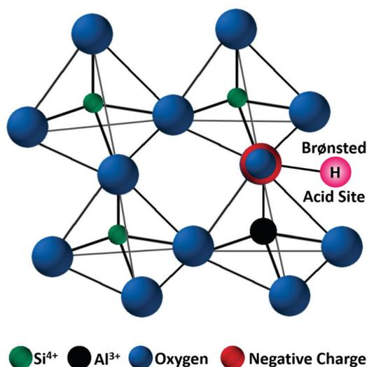
Fig. 5 Representative zeolite framework of a tetrahedral  $[SiO_4]^{4-}$ , with generation of a negative charge due to the incorporation of  $Al^{3+}$  and substitution of a proton to maintain the charge balance. Adapted with permission from ref. 45. Copyright (2002) Elsevier.
