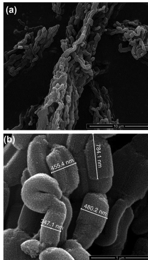
Fig. 20 SEM images of SBA-15-SO<sub>3</sub>H catalyst. Reproduced with permission from ref. 196. Copyright (2014) John Wiley and Sons.
