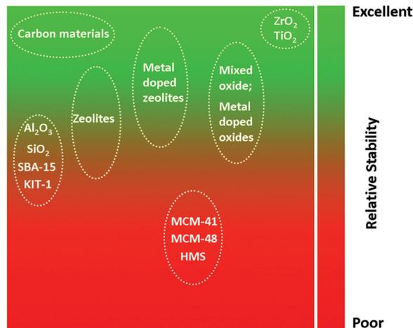
Fig. 26 Hydrothermal stability of different heterogeneous solid catalysts in superheated steam conditions ( $T > 400$  °C). Reproduced with permission from ref. 284. Copyright (2014) Royal Society of Chemistry.
