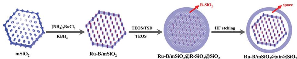
Fig. 19 Illustration of the synthesis process of yolk-shell structured Ru–B/mSiO<sub>2</sub>@air@SiO<sub>2</sub> catalyst. Reproduced with permission from ref. 192. Copyright (2014) American Chemical Society.
