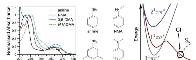
Fig. 1 The vapour phase spectra of aniline (black line), NMA (red line), 3,5-DMA (blue line), and N,N-DMA (green, dot-dashed line) are shown on the left with the corresponding structures shown in the middle panel. A schematic potential energy cut along the aniline N-X reaction coordinate is shown on the right (adapted from ref. 16).
