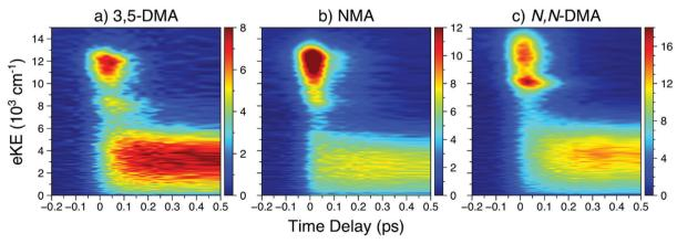
Fig. 2 In order of increasing amine substitution, the short time delay TR-PES results at  $\lambda_{pu} = 238$  nm and  $\lambda_{pr} = 305$  nm from (a) 3,5-DMA, (b) NMA, and (c) N,N-DMA.
