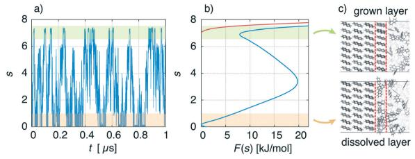
Fig. 5 a) Time evolution of the biased CV, s. The orange shaded region relates to the dissolved crystal layer, while the green shaded region corresponds to the grown layer. b) Corresponding FES, F(s) (blue curve), and wall potential (red curve). c) Representative simulation box snapshots of states at each minimum of the FES.
