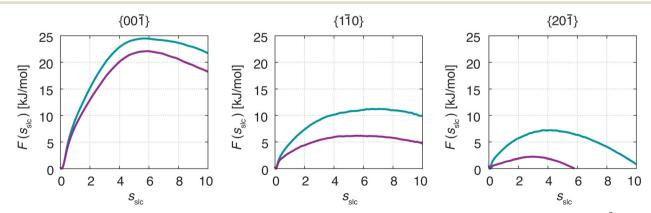
Fig. 6 Free energy,  $F(s_{slc})$ , in dependence of crystallinity of the crystal surface,  $s_{slc}$ . Green denotes the concentration at  $C = 1.2 \text{ nm}^{-3}$ , and purple denotes the concentration at  $C = 1.5 \text{ nm}^{-3}$
