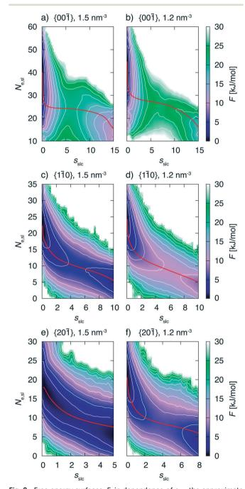
**Fig. 8** Free energy surfaces, F, in dependence of  $s_{\rm slc}$ , the approximate number of crystalline naphthalene molecules in the surface layer, and  $N_{\rm e,sl}$ , the number of ethanol molecules in the surface layer. The white isocontours are drawn in 2.5 kJ mol $^{-1}$  energy steps. The red lines correspond to the minimum free energy paths. Fig. 8a)–f) show the free energy surfaces for different faces and supersaturations.
