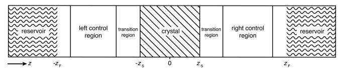
Fig. 1 Schematic of the  $C_{\mu}MD$  method illustrating the segmentation of the simulation box. The two crystal surfaces are perpendicular to the z-axis and exposed to the solution at positions  $-z_S$ , and  $z_S$  respectively. The external force positions are marked at  $-z_F$  and  $z_F$ .
