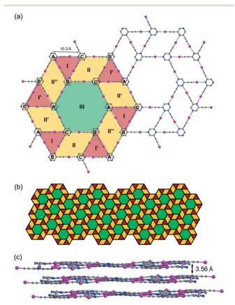
Fig. 5 (a) Projection diagram showing the tacit trihedral snub trihexagonal tessellation stabilized by C-I···N halogen bonds with three independent L2 molecules in L2b. (b) Schematic diagram showing the pattern of the complete tessellation of a single layer in L2b. (c) Projection diagram showing the stacking of the tiling layers in the crystal structure. All hydrogen atoms are omitted for clarity.
