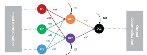
Fig. 2 Schematic graph showing a MLP type ANN with 3 normalised input parameters (IL), all connected with weights (wXX) to the hidden neuron layer (HL) which in turn is connected with weights to the single output neuron (OL). Outputs from the hidden and output layers are modified by biases (bX). The final output is then denormalised.
