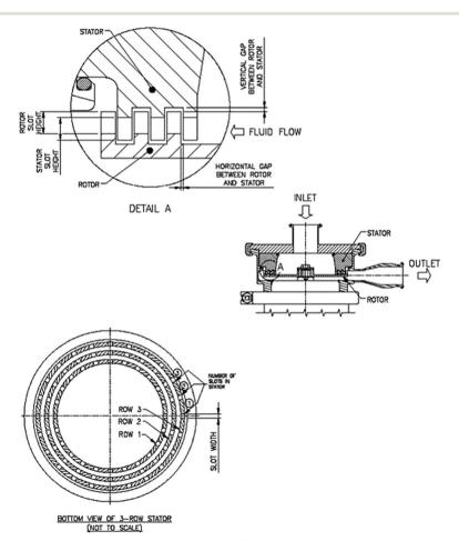
Fig. 7 Schematic view of the tooth geometry of a typical rotor-stator mill.<sup>124</sup> The slots in the rotor and stator and their heights can vary. Reprinted with permission from ref. 124, Copyright 2013 American Chemical Society.
