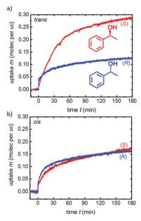
Fig. 3 Enantiopure uptakes of (R)- and (S)-phenylethanol by the Cu<sub>2</sub>(DCam)<sub>2</sub>(AzoBiPyB) film in the trans state (a) and cis state (b). The uptake is determined with a guartz crystal microbalance (QCM) in combination with a gas flow system. The molecular structures of (R)- and (S)-phenylethanol are sketched in the inset in (a)
