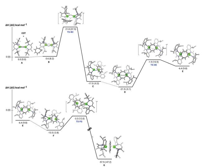
DFT (B3PW91) computed enthalpy reaction profile at room temperature for the reaction of compound 2 (A) and 1,3,5,7-C<sub>8</sub>H<sub>8</sub>
