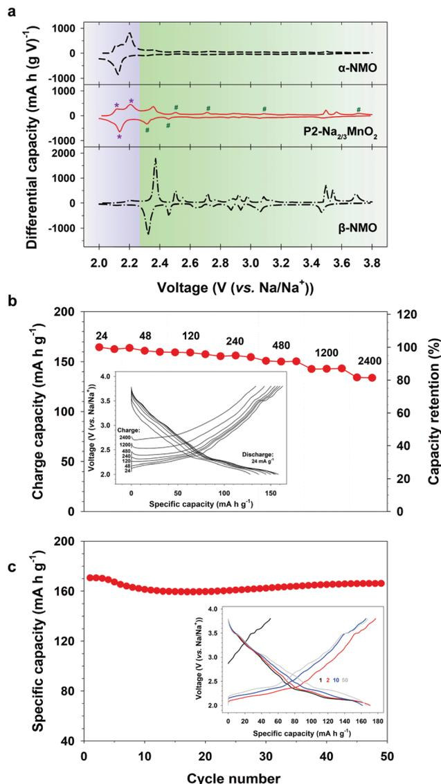
Fig. 4 Sodium storage performance of the nanostructured P2-Na<sub>2/3</sub>MnO<sub>2</sub>. (a) Differential capacity plots at 12 mA g<sup>-1</sup>. Data for α-NMO and β-NMO were adapted from ref. 32. (b) Rate performance at various charge current densities. (c) Cycling performance at 12 mA g<sup>-1</sup> (inset: corresponding voltage profiles).
