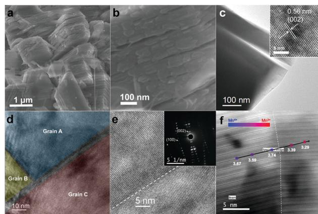
Fig. 3 (a) and (b) SEM images and (c) TEM image of the nanostructured P2- $\text{Na}_{2/3}\text{MnO}_2$  (Inset: Magnified HRTEM image). HRTEM images of (d) three neighboring grains: A, B, and C (e) the interface region with a SAED pattern (inset) indicating the different orientations. (f) High-angle annular dark-field STEM image of the interface region with an EELS line scan.
