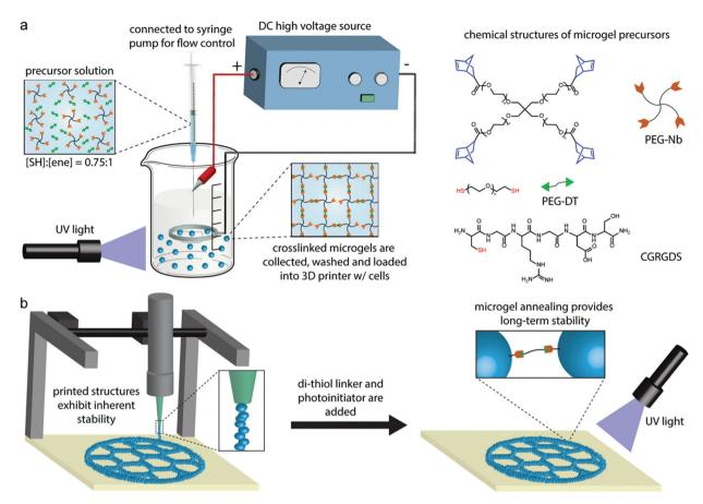
Fig. 1 Overview of clickable PEG microgel bioink production and use in 3D printing. (a) Chemical structures and schematic of the submerged electrospraying setup for synthesizing PEG microgels *via* thiol—ene click chemistry. (b) Schematic of PEG microgel 3D printing procedure. Printed structures exhibit inherent stability due to the cohesive forces between PEG microgels. Long-term stability is achieved by annealing the microgels with a second thiol—ene reaction that crosslinks the microgels.
