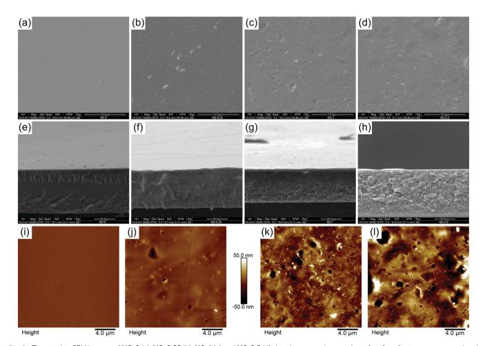
Fig. 6 Top section SEM images of M2-0 (a), M2-0.25 (b), M2-1 (c) and M2-2.5 (d) showing a growing number of surface features; cross-sectional SEM images of M2-0 (e), M2-0.25 (f), M2-1 (q) and M2-2.5 (h) showing a more grainy texture; AFM height images of M2-0 (i), M2-0.25 (j), M2-1 (k) and M2-2.5 (I) showing a higher surface roughness with increasing amount of mGO-1 loading.
