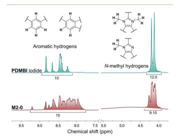
Fig. 5 <sup>1</sup>H NMR spectra of PDMBI iodide and M2-0 membrane showing aromatic and N-methyl hydrogens. The area ratios of the signals show 100% and 50-60% quarternisation of the benzimidazole groups for PDMBI and M2-0, respectively.
