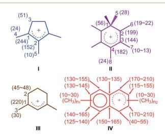
Fig. 2 Carbocations identified in activated M-β and MMM-β coded with the same colors as their corresponding assignments and correlations in Fig. 3 and 4. Values in the parenthesis are  $^{13}$ C chemical shifts.  $n_1$  and  $n_2$  are the number of methyl groups with  $3 \le (n_1 + n_2) \le 7$ .
