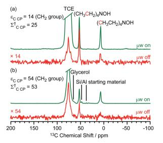
Fig. 1  $^{13}$ C CP MAS DNP spectra of templated (a) M- $\beta$  and (b) MMM- $\beta$  with ( $\mu$ w on) (green) and without ( $\mu$ w off) microwave irradiation (red) at 9.4 T. TCE stands for 1,1,2,2-tetrachloroethane (solvent of impregnation).
