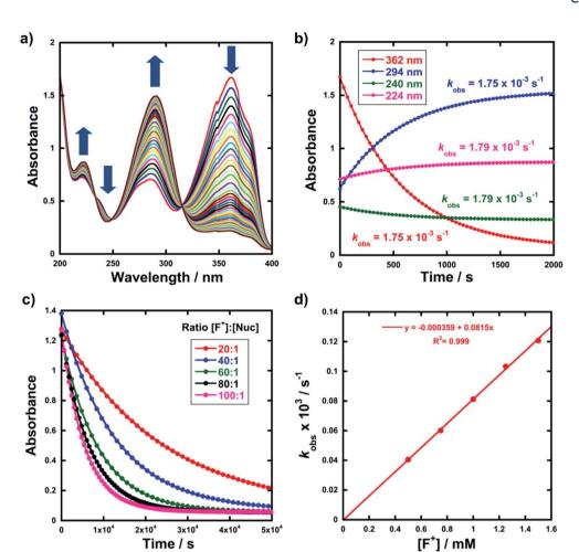
Fig. 2 (a) UV-vis spectra during the reaction of 1d (0.05 mM) with Selectfluor<sup>TM</sup> (in CH<sub>3</sub>CN at 25 °C), each spectrum acquired at 30 s intervals. The shoulders at 350 nm are artefacts that correspond to the spectrophotometer switching from UV to VIS lamps. (b) Exponential behaviour at 4 different wavelengths. (c) Representative exponential decays of absorbance with different concentrations of  $F^+$ . (d) Representative correlation of  $k_{\text{obs}}$  with  $[F^+]$ .
