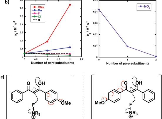
Fig. 6 (a) Eyring plots for fluorination of 1,3-dicarbonyls 1a-e by Selectfluor<sup>TM</sup> 3 in CH<sub>3</sub>CN at 20 °C, 25 °C, 30 °C and 35 °C, and associated activation parameters. (b) Effect of mono- vs. di-substitution on the rate of fluorination; all rate constants were obtained in CH<sub>3</sub>CN at 25 °C. (c) Asymmetry of the enol in the transition state.
