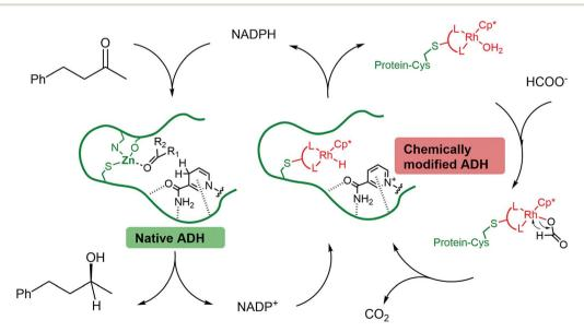
Fig. 1 Reduction of a model ketone using a native-artificial enzyme cascade with the same alcohol dehydrogenase scaffold. L-L represents a bidentate ligand. The protein is represented in green, and the rhodium complex is represented in red.
