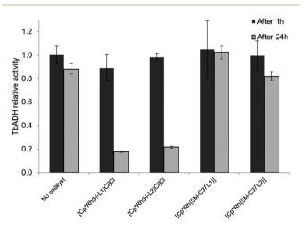
Fig. 5 Effect of the free and bioconjugated rhodium catalysts on 2butanone reduction by WT TbADH. WT TbADH (1 μM) was incubated with the corresponding Rh catalyst (5 μM) in sodium phosphate buffer (100 mM, pH 7). In the absence of the Rh catalyst, the specific activity of WT TbADH (2-butanone reduction coupled to NADPH oxidation) after 1 h heating was 4.95  $\pm$  0.37 U mg<sup>-1</sup>
