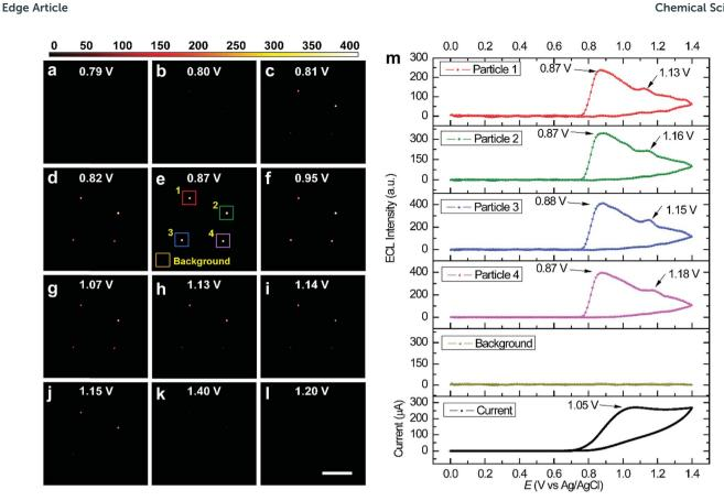
Fig. 2 (a-I) Successive ECL snapshots of four RuDSNs during a potential cycle. Scale bars (white), 30 μm. (m) ECL intensity of four nanoparticles and blank area in (e) as a function of electrode potential and the corresponding CV curve of the GC electrode (black line) recorded by the potentiostat. The potential was cyclically scanned from 0 to 1.4 V at a scan rate of 20 mV s<sup>-1</sup> in 200 mM PBS buffer containing 100 mM TPA. The exposure time of EMCCD was 500 ms.
