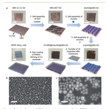
Fig. 1 Fabrication and SEM characterization of the SERS sticky note: (a) Optical images and schematic illustration of the step-by-step fabrication process of the SERS sticky note by self-assembly of DDT, IAUNSs and sAUNSs on hBN, encapsulation with IS-implanted hBN, spin-coating of PMMA, and etching of the Cu substrate. Scale bars: 2 mm. (b and c) SEM images of the SERS sticky note with scale bars of (b) 2  $\mu$ m and (c) 200 nm.
