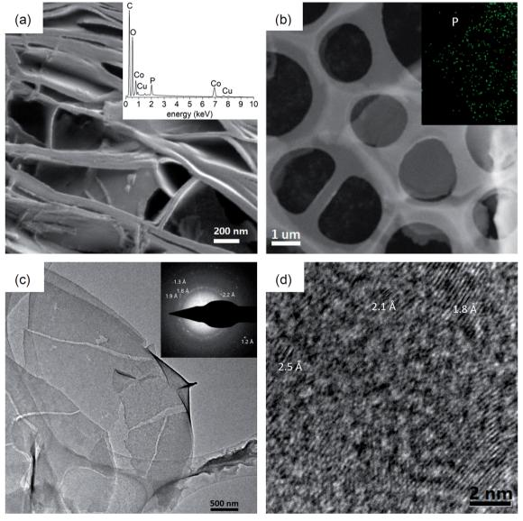
Fig. 5 (a) SEM image and the EDX spectrum (inset) of an irradiated MOFs@P4 with partial exfoliation; (b) SEM image of a thin sheet and the EDX mapping of the P element (inset); (c) TEM image and SAED spectrum (inset) of thin sheets; (d) HRTEM image of the thin sheet.
