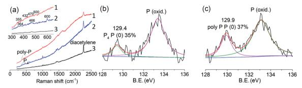
Fig. 4 (a) Raman spectra of the MOF (curve 1), MOFs@P<sub>4</sub> (curve 2) and irradiated MOFs@P<sub>4</sub> (curve 3), respectively; (b) XPS spectrum of the P 2p envelope of MOFs@P4; (c) XPS spectrum of the P 2p envelope of irradiated MOFs@P4.
