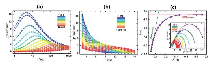
Fig. 5 Magnetic properties of II. (a) Frequency and (b) temperature dependence of the out-of-phase ac-susceptibilities. (c) Arrhenius plots of the relaxation rate and its fitting (see the text); inset: Cole-Cole plot and fits at different temperatures.
