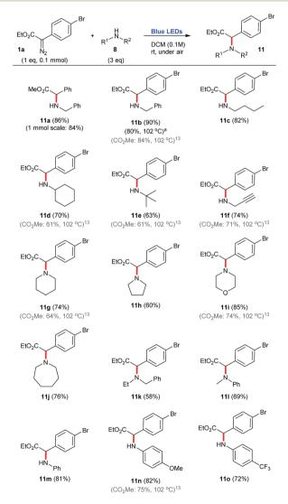
Scheme 4 N–H insertion reactions employing aryldiazoacetate 1a and a number of amines, under blue light irradiation. <sup>a</sup>Prepared under thermal conditions. <sup>13</sup>
