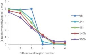
Fig. 5 Concentration profiles of (top) hexylamine and (bottom) 1-naphthylmethylamine between regions 1 and 6 of the diffusion cell. At the start of the experiment, hexylamine is loaded in regions 4–6 of the diffusion cell and 1-naphthylmethylamine is loaded in regions 1–3. As time progresses, the concentrations of the amines change as diffusion leads to exchange across the gel–gel interface. The points in these graphs are joined together solely as a guide to the eye.
