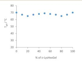
Fig. 8 Thermal stability of mixtures of enantiomeric L-Lys-HexGel and D-Lys-HexGel at a total concentration of 10 mM, as determined using tube inversion methodology.
