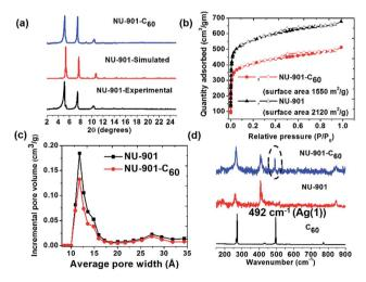
Fig. 2 (a) PXRD pattern of simulated NU-901, experimental NU-901, and experimental NU-901- $C_{60}$ , (b)  $N_2$  adsorption–desorption isotherms (77 K) (NU-901 and NU-901- $C_{60}$ ), (c) density functional theory (DFT) pore size distribution (NU-901- $C_{60}$  and NU-901) and, (d) Raman spectra (NU-901, NU-901- $C_{60}$  and  $C_{60}$ ).
