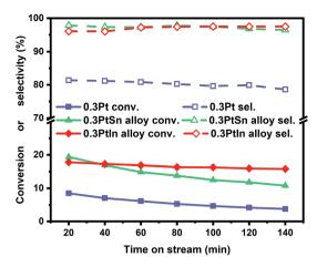
Fig. 4 The conversion and selectivity of Pt, Pt<sub>3</sub>In and Pt<sub>3</sub>Sn catalysts in the propane dehydrogenation process ( $T=600\,^{\circ}$ C, atmospheric pressure, WHSV = 3 h<sup>-1</sup>, C<sub>3</sub>H<sub>8</sub>/H<sub>2</sub> = 1:1, the total flow rate is 50 mL min<sup>-1</sup> with N<sub>2</sub> balanced).
