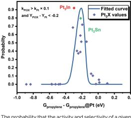
Fig. 3 The probability that the activity and selectivity of a given catalyst are better than pure Pt under given activity and selectivity constraint conditions as a function of propylene adsorption energy relative to that of Pt (Y: the difference between propylene desorption free energy barrier and further dehydrogenation step free energy barrier of Pt<sub>3</sub>X,  $k_{\text{Pt-X}}$ : the rate constants of Pt<sub>3</sub>X).
