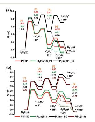
Fig. 5 (a) Gibbs free energy diagram of  $\alpha$ -type ( $C_3H_8 \rightarrow 1$ - $C_3H_7^* \rightarrow$  $C_3H_6^* \rightarrow 1-C_3H_5^*$ ) PDH reaction on Pt(211), Pt<sub>3</sub>In(211)\_Pt and Pt<sub>3</sub>In(211) In. (b) Gibbs free energy diagram of  $\alpha$ -type PDH reaction on Pt(111),  $Pt_3In(111)$ ,  $Pt_1In_1(111)$  and  $PtIn_2(110)$ .
