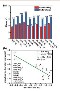
Fig. 6 (a) The d-band filling and Bader charge analysis. (b) Correlation between the d-band center of surface Pt and propylene  $\pi$  adsorption energy.
