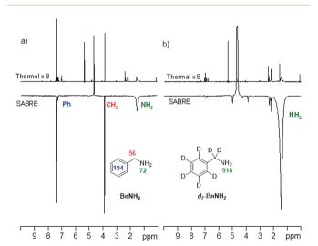
Fig. 2 (a) <sup>1</sup>H NMR spectra of BnNH<sub>2</sub>, thermally polarised, top, and hyperpolarised, bottom. (b)  $^{1}H$  NMR spectra for  $d_{7}$ -BnNH<sub>2</sub>, thermally polarised, top, and hyperpolarised, bottom.
