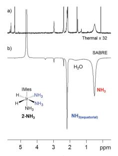
Fig. 1 (a) The thermally polarised  $^1H$  NMR SABRE spectrum ( $\times$  32 vertical expansion) recorded of 2-NH3 (formed by reaction of 1 with  $NH_3$  and  $H_2$ ) in dichloromethane- $d_2$  at 298 K. (b) The corresponding SABRE polarised 9.4 T  $^{1}$ H NMR spectrum after transfer under p-H $_{2}$  at 60 G. The hyperpolarised responses of free NH<sub>3</sub> and Ir-NH<sub>3(equatorial)</sub> of 2-NH<sub>3</sub> and residual H<sub>2</sub>O are indicated.
