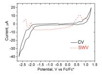
Fig. 6 Cyclic (CV) and square wave (SWV) voltammograms of 1 (1 mM) in THF (internal standard Fc/Fc\*,  $v=0.1~\rm V~s^{-1}$ ).
