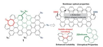
Fig. 1 Key structural features (right) present in the target distorted ribbon-shaped graphene molecule 1 (left).
