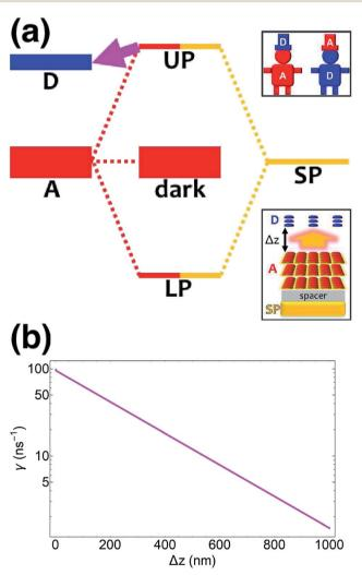
Fig. 3 (a) Schematic energy-level diagram showing the "carnival-effect"-EET role-reversal process from acceptor UP state to bare donors. Insets: (top) cartoon illustrating the "carnival effect" between donors and acceptors and (bottom) representation of the reversed-role EET process from a thick and dense slab of acceptors (featuring SC to SPs) to a dilute monolayer of donors. (b) Rate as a function of donor–acceptor separation  $\Delta z$  for energy transfer from acceptor UP to bare donors.
