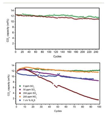
Fig. 6 (Top panel) Long-term CO<sub>2</sub> adsorption performance stability of PEI/(Zn)ZIF-8/SiO<sub>2</sub> (green) and PEI/(Zn)ZIF-7/SiO<sub>2</sub> (dark red) under simulated flue gas conditions. (Bottom panel) Long-term CO<sub>2</sub> adsorption performance stability of PEI/(Zn)ZIF-8/SiO $_2$  under the presence of SO<sub>2</sub>, NO<sub>x</sub> and H<sub>2</sub>S contaminants.
