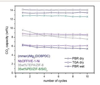
Fig. 3 CO<sub>2</sub> capture of polyamines impregnated on bulk MOFs compared with MOF/SiO2 under simulated flue gas conditions in a PBR.
