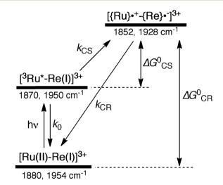
Scheme 2 Photoexcitation and the subsequent relaxation processes of a  $[Ru(ii)-Re(i)]^{3+}$  binuclear complex in the absence of any quencher molecules in solution, *i.e.*, the formation of a triplet metal-to-ligand charge transfer excited state  $([^3Ru^*-Re(i)]^{3+})$  followed by a charge-separated state  $([^4Ru)^*-(Re)^*-]^{3+})$  due to electron transfer from the Ru unit to the Re unit. Wavenumber values shown are for the RuRe(OEt) complex.
