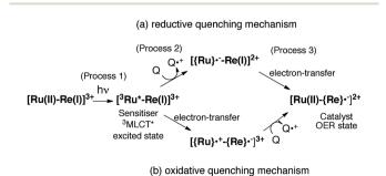
Scheme 1 Reductive and oxidative pathways in the photochemical formation of the OERS of RuRe(X).
