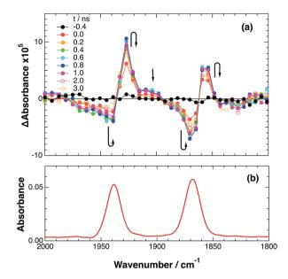
Fig. 5 (a) TRIR spectra (ps-system) recorded after 532 nm excitation of RuRe(FPh) (1 mM) in an argon-saturated CH<sub>3</sub>CN solution. (b) FT-IR spectrum of RuRe(FPh) in CH<sub>3</sub>CN.
