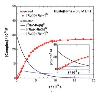
Fig. 7 Time profile of  $[Ru(\shortparallel)-\{Re\}^{\cdot-}]^{2+}$  (•) in the ps-TRIR measurement of RuRe(FPh) in the presence of 0.3 M BIH in an argon-saturated DMF-TEOA (5 : 1 v/v) solution after 532 nm excitation. The kinetic simulation results for  $[^3Ru*-Re(\shortparallel)]^{3+}$ ,  $[\{Ru\}^{\cdot-}-Re(\shortparallel)]^{2+}$ , and  $[Ru(\shortparallel)-\{Re\}^{\cdot-}]^{2+}$  are also shown (solid lines).
