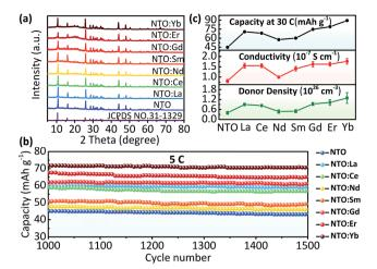
Fig. 4 (a) The powder XRD patterns of NTO and NTO:Ln (Ln = La, Ce, Nd, Sm, Gd, Er, and Yb). (b) The cyclic performance of NTO and NTO:Ln at the current rate of 5C with the number of cycles ranging from 1000 to 1500. (c) The overview of capacities, electron conductivities and donor densities of NTO and NTO:Ln.
