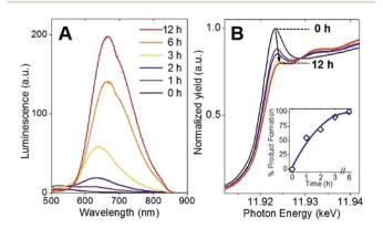
Fig. 4 (A) Photoluminescence spectra (excitation  $\lambda=470$  nm) and (B) Au L<sub>3</sub>-edge XANES (inset, white-line integration analysis for Au(III) to Au(I) formation) following the course of the protein-directed assembly of Au clusters.
