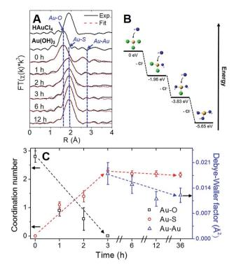
Fig. 5 (A) Au  $L_3$ -edge FT-EXAFS with fitted spectra and reference materials. (B) Relative DFT energies of AuCl $_3$  (set to 0 eV), Au(OH) $_3$ , and intermediate products of the precursor ion-exchange process. (C) Coordination and Debye–Waller (Au–Au shell only) plot for time-dependent EXAFS fitting results.
