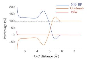
Fig. 3 Top panel: the PES of a water trimer when one water is pulled away from the other two. Bottom panel: the percentage contribution of the Behler–Parrinello atom-wise energy, electrostatic energy and van der Waals energy to the binding energy between the water that is pulled away and the other two waters. The Behler–Parrinello atomwise energy contributes most of the binding energy at short range and the electrostatic energy is the dominant contribution at long range.
