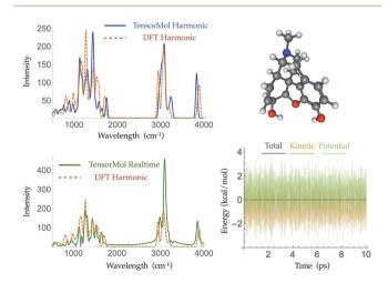
Fig. 7 The geometry of morphine as optimized by TensorMol-0.1 (upper right panel) and its harmonic IR spectra simulated using  $\omega B97X-D/6-311G^{**}$  (dashed orange line) and the TensorMol force field (solid blue line) (upper left panel). The lower panels show the real-time IR spectra obtained using TensorMol (solid green line), and the DFT results (dashed orange line) (left), and the conservation of energy maintained by the smoothness of the energy (right).
