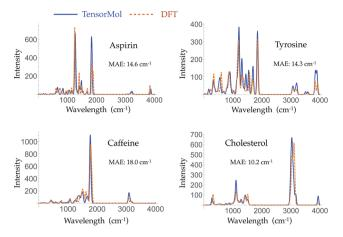
Fig. 8 Harmonic IR spectra of four different molecules simulated using  $\omega$ B97X-D/6-311G\*\* (dashed orange line) and TensorMol-0.1 (solid blue line). All these molecules were not included in the training set.
