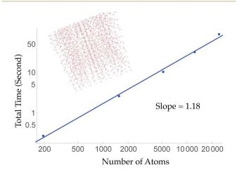
Fig. 2 Aperiodic timings of an energy, charge and force call for cubic water clusters at a density of 1 g cm<sup>-3</sup>. The largest  $\sim$ 60 Angstrom cube is 4× larger than the electrostatic cutoff. The slope of a log-log version of this curve is near unity, indicating the wall-time scaling of TensorMol. Inset figure: the cubic water cluster used for timing containing 1728 water molecules
