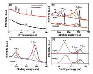
Fig. 3 (a) XRD patterns of V-Co(OH)F/CC and V-CoP/CC. XPS spectra in the (b) Co 2p, (c) V 2p, and (d) P 2p regions for V-CoP/CC and CoP/CC.
