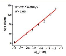
Fig. 4 Variance of Cy5 counts with different-concentration methylated DNA. The Cy5 counts exhibit a linear correlation with the logarithm of methylated DNA concentration in the range from 1  $\times\,10^{-18}$  to  $1\times10^{-11}\,\text{M}.$  The concentration of each DNA probes X, Y, X' and Y' is 1.0 imes 10<sup>-6</sup> M. The concentration of 605QD is 8.3 nM. Error bars show the standard deviation of three experiments.
