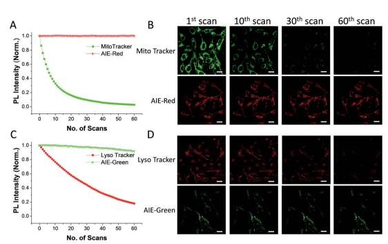
Fig. 2 Relative fluorescence intensities of AIE-Red (A, red), Mito Tracker (A, green), AIE-Green (C, green) and Lyso Tracker (C, red) under continuous scanning; confocal images of HeLa cells stained with AIE-Red (B, lower panel), Mito Tracker (B, upper panel), AIE-Green (D, lower panel) and Lyso Tracker (D, upper panel) after being scanned various times. The scale bar is 20 μm.
