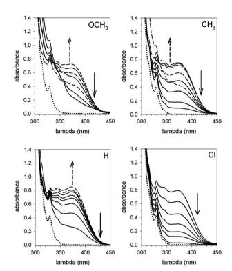
Fig. 3 Time dependent UV-vis spectra of the reaction mixtures composed of equimolar amounts (0.30 mM) of catenane 1 and acid 2 (X = OCH $_3$ , CH $_3$ , H and Cl) in CH $_2$ Cl $_2$  at 25 °C. The dotted lines represent the absorption spectrum of 1. The spectra pictured as broken lines refer to the ascending phase of the absorbance, whereas the full lines refer to the descending phase.
