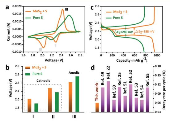
Fig. 5 (a) CV curves, (b) discharge-charge curves and (c) the comparison of the peak voltages of the pure S and  $MoS_2 + S$  electrodes. (d) A comparison of the decay rate per cycle with that of other Li-S cathode materials reported in the literature recently.
