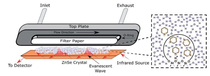
Fig. 2 Schematic of an ATR flow cell. Inset: Depiction of the pyridine partition (concentration change) between the bulk solvent and the pores detected *via* ATR-FTIR.
