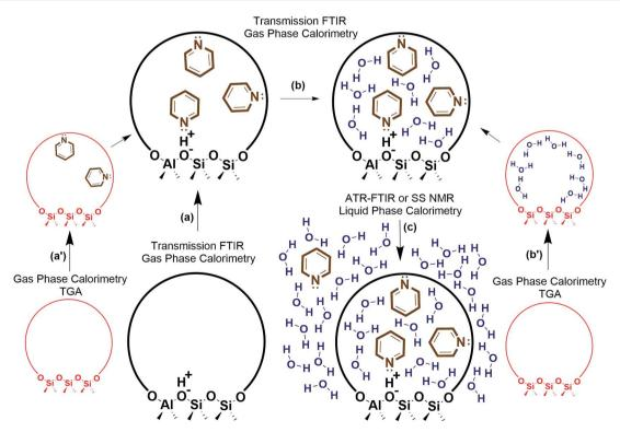
Experimental outline for estimating liquid phase adsorption, solvation, and interaction energies
