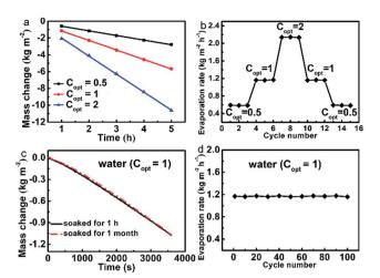
Fig. 3 Durability and stability of the evaporator. (a) The evaporation mass changes of water under different  $C_{\rm opt}$  within 5 hours. (b) The evaporation cycle performance of the evaporator under different solar concentrations. (c) Evaporation rate curves of the evaporator soaked in water after 1 h and 1 month. (d) The evaporation cycle performance of the evaporator in water over 100 cycles, with each cycle sustained for 1 h
