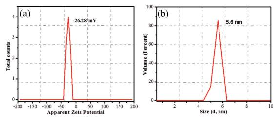
Fig. 1 Zeta potential (a) charge of GSH-CDs, (b) hydrodynamic diameter of GSH-CDs.
