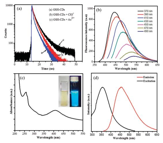
Fig. 5 (a) Fluorescence decay curves of GSH-CDs (blue colored curve (a)), GSH-CDs with ClO- (red colored curve (b)), and GSH-CDs with As<sup>3+</sup> (black colored curve (c)). (b) Excitation-dependent fluorescence emission of GSH-CDs with excitation from 370 to 490 nm. (c) UV-vis absorption spectra of GSH-CDs. The inset image is an aqueous dispersion of GSH-CDs in day light and UV light, respectively. (d) Fluorescence excitation and emission response of the GSH-CDs.
