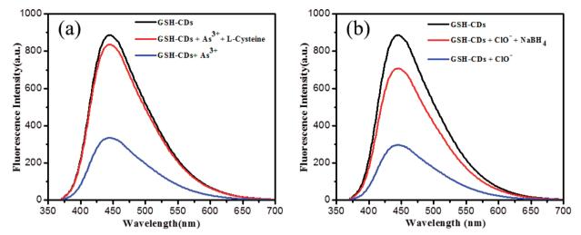
Fig. 11 (a) Fluorescence response 10  $\mu$ L of GSH-CDs for As<sup>3+</sup> ions (25 nM) and recovery of L-cysteine. (b) Fluorescence response of GSH-CDs for CIO<sup>-</sup> ions (100  $\mu$ M) and the recovery of NaBH<sub>4</sub>.
