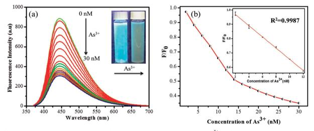
Fig. 7 (a) Fluorescence emission response of 10  $\mu$ L GSH-CDs, to various molar equivalents of As<sup>3+</sup> ions (0 to 30 nM) in 1000  $\mu$ L of tris-HAc buffer (10 mM, pH 7.4). (b) Stern-Volmer plot with an inset plot shows the linearity for As<sup>3+</sup> ions (2 to 12 nM).
