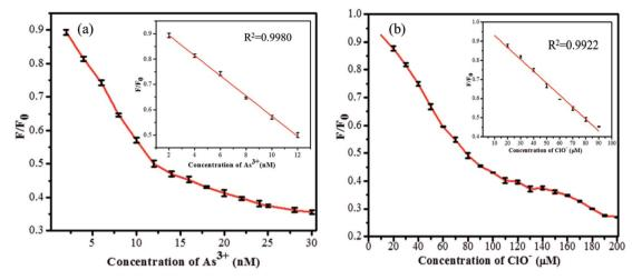
Fig. 12 (a) Fluorescence response of GSH-CDs for  $As^{3+}$  ions (0–30 nM) in tap water, (b) for  $ClO^-$  ions (0–200  $\mu$ M) in tap water. The triplicated data were fitted in the linearity equation of  $F_0/F$  for tap water sample analysis, shown as in insert image.
