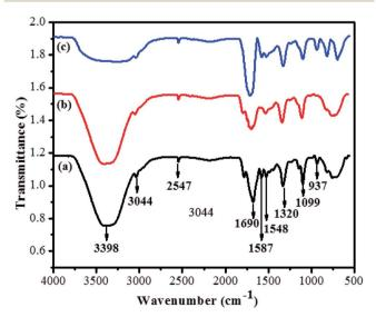
Fig. 4 (a) FTIR patterns of GSH-CDs, (b) with  ${\rm As}^{3+}$  and (c) with ClOions.
