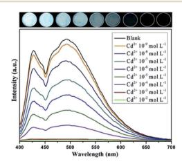
Fig. 5 Fluorescence responses of complex with Cd<sup>2+</sup>metal ion with different concentrations (excited at 365 nm).
