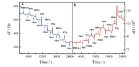
Fig. 3 Response in frequency (a) and dissipation (b) for fabrication process of quartz/PDDA-G/(PSS/PDDA)3/CDs SAMs.
