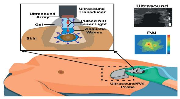
Fig. 7 Integrated real-time photoacoustic/ultrasound imaging
