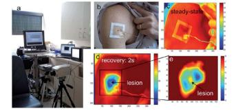
Fig. 14 (a) The infrared imaging system, (b) photograph of the body surface area with a cluster of pigmented lesions, (c) reference infrared image of the region at ambient temperature, (d) the same area after cooling and (e) magnified section of the melanoma lesion and surroundings. Reproduced under CC license from ref. 19.
