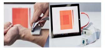
Fig. 15 sKan device. This device detects skin cancer using thermal images that are obtained from affected areas of the skin surface using thermistors. Reproduced from ref. <sup>202</sup>.
