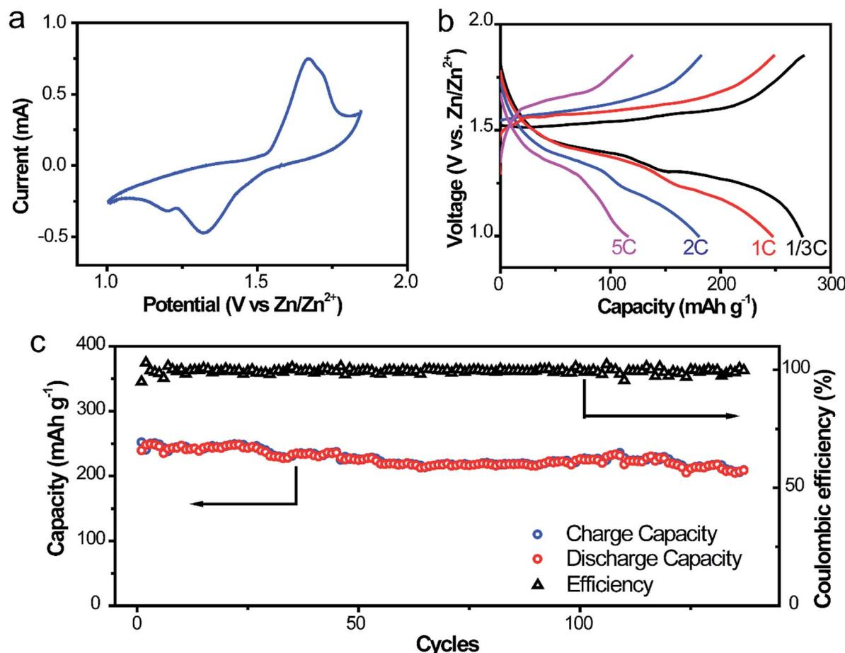
Fig. 6 (a) CV scanning profile at 0.5 mV s<sup>-1</sup> (b) galvanostatic discharging/charging profiles at 1/3, 1, 2, 5C rate, respectively. (c) Cycling performances of Zn@CFs| $\alpha$ -MnO<sub>2</sub> full cell at 1C rate.
