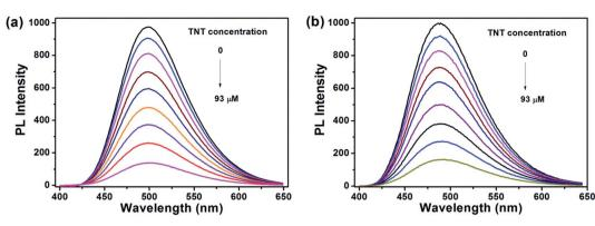
Fig. 3 PL spectra of (a) PTPA1-TPE and (b) PTPA2-TPE in 9:1 (v/v) water/THF solution containing different amounts of TNT. Polymer concentration:  $10^{-5}$  M.
