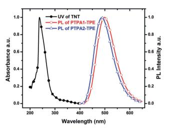
Fig. 4 Normalized absorption spectrum of TNT in THF solution and PL spectra of PTPA1-TPE and PTPA2-TPE nanoaggregates in 9:1 (v/v) water/THF dispersion.
