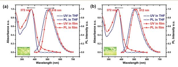
Fig. 1 Normalized absorption and PL spectra of (a) PTPA1-TPE and (b) PTPA2-TPE in dilute THF solution ( $10^{-5}$  M) and as spin-coated films (measured at room temperature). The insets in (a) and (b) show fluorescent images of PTPA1-TPE and PTPA2-TPE powders under UV irradiation, respectively.
