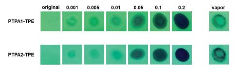
Fig. 7 Paper test strips impregnated with PTPA1-TPE or PTPA2-TPE before and after dropping TNT solutions in THF onto them (concentration: 0.001, 0.005, 0.01, 0.05, 0.1 and 0.2 mg mL $^{-1}$ , respectively), and after storage above TNT vapor for 5 min.
