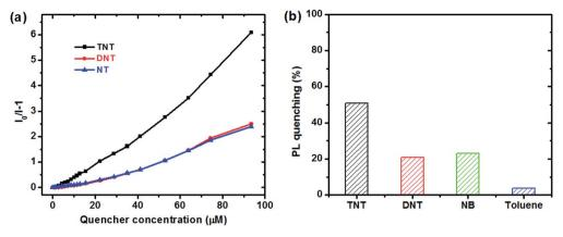
Fig. 6 (a) Stern-Volmer plots of the relative PL intensities of PTPA1-TPE ( $I_0/I - 1$ ) vs. concentration of the analytes TNT, DNT and NB (I: PL intensity,  $I_0$ : PL intensity at zero analyte concentration). (b) PL quenching of PTPA1-TPE for analyte concentrations of 22  $\mu$ M.
