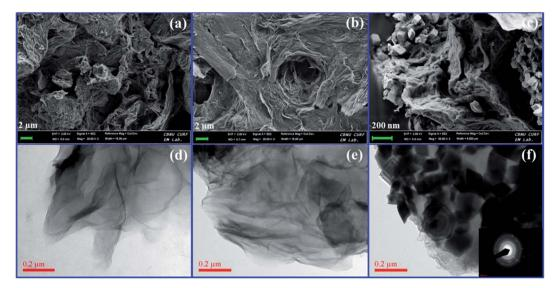
Fig. 1 FE-SEM images of (a) GO, (b) SGO and (c) Fe<sub>3</sub>O<sub>4</sub>–SGO; TEM images of (d) GO, (e) SGO and (f) Fe<sub>3</sub>O<sub>4</sub>–SGO and inset (f) SAED pattern.
