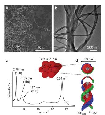
Fig. 5 (a and b) SEM (a) and TEM images (b) of nanofibers of 3 (c = $5.0 \times 10^{-5}$  M) obtained from THF/water = 50:50 (v/v) solutions. (c) The XRD pattern of nanofibers (values in parentheses denote Miller indices). (d) A schematic model for the hexagonal molecular packing of helically stacked 3
