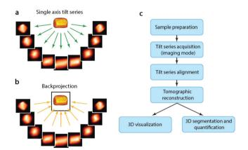
Fig. 7 (a) A tilt series of images of a 3D object are recorded as projections and (b) then back-projected to retrieve the 3D volume. (c) Steps involved in an ET experiment from sample preparation to 3D visualization and quantification.41
