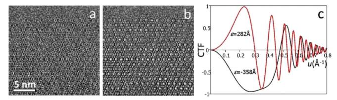
Fig. 2 HRTEM images of ITQ-39 taken along the [100] axis at defocus 282 Å (a) and -358 Å (b). Image (b) was taken close to the Scherzer defocus, therefore atomic columns are shown as black dots. The contrast transfer functions of (a) and (b) are shown in (c).
