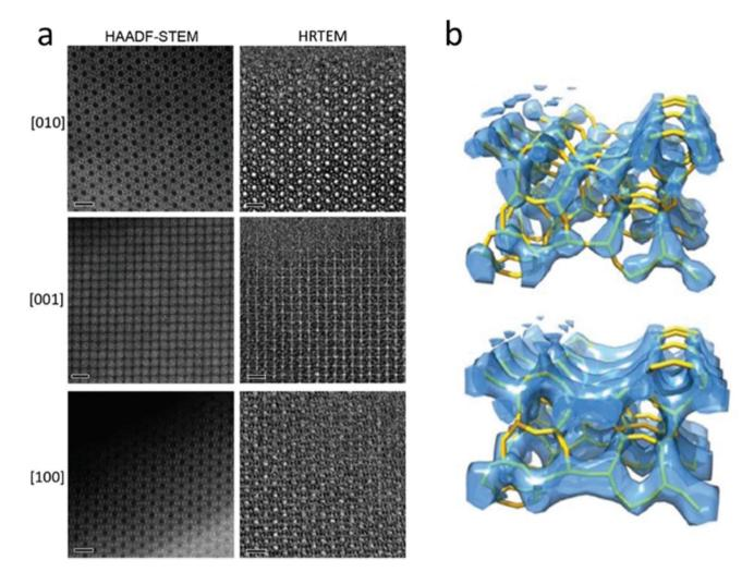
Fig. 4 (a) Aberration-corrected HAADF-STEM images (left) and HRTEM images (right) of zeolite silicalite-1 taken along the three main zone axes [010], [001] and [100]. The scale bars are 2 nm. Note that the contrast is reversed between the HAADF-STEM and the HRTEM images. The pores are black in the HAADF-STEM images and white in the HRTEM images. (b) Reconstructed 3D map from the HAADF-STEM images (top) and the HRTEM images (bottom), with the structure model inserted. 17
