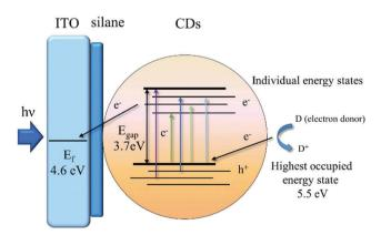
Fig. 4 The mechanism of photoelectric conversion of CDs.
