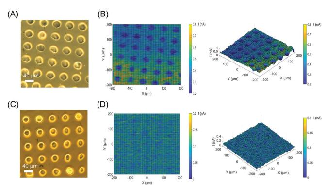
Fig. 5 (A) Optical micrograph of a PMMA dot array on the ITO-silane-CD surface obtained by microcontact printing; (B) the corresponding ac-photocurrent image of (A) measured at 1.8 V; (C) the optical micrograph of a PMMA dot array on the ITO-silane surface; (D) the corresponding ac-photocurrent image of (C) measured at 1.8 V.
