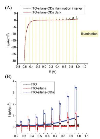
Fig. 3 (A) LSV curves of ITO-silane-CDs in the dark and with chopped illumination (420-450 nm, 10 mW cm<sup>-2</sup>, a UV blocking filter was used to block light at wavelengths < 420 nm); (B) LSV curves of ITO, ITO-silane, and ITO-silane-CDs with chopped illumination.
